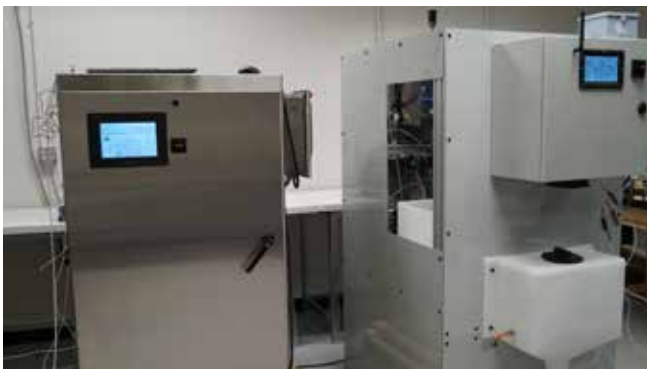
Figure 2: Plasma/copper-silver ionization unit and oxidizing biocide generator.
