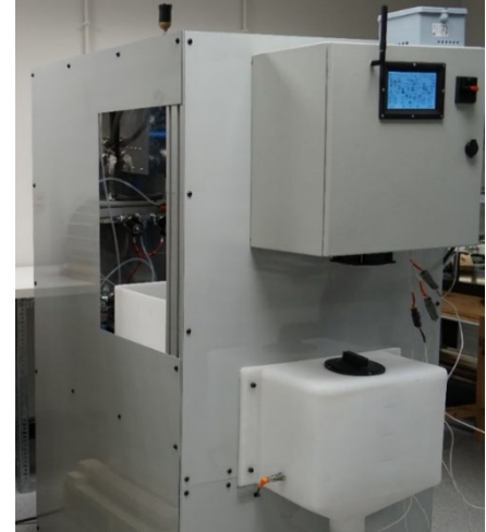
Figure 3 – Electrolyzer - Oxidizing Biocide Generator
